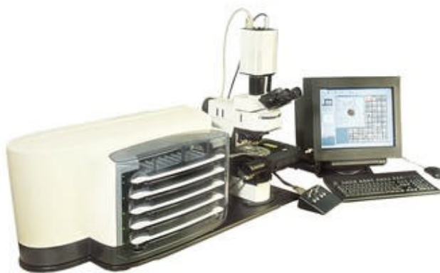
Figure 7. Ariol SL-50 is a complete slide digitization and image analysis system, with plenty of modules for immunohistochemistry and tissue microarrays.
